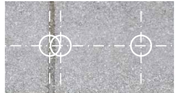
Individual positioning of the fastener - close to, or even right on a low between two highs - without shimming
